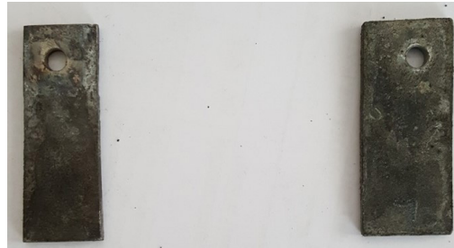
Figure 5: ConduCrete Pro encased Samples, Bare Steel (left) and Galvanized Steel (right), after Experiment
